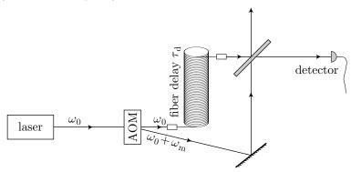
The fiber is assumed to cause a well-defined time delay of the undiffracted beam, of around 5  $\mu$ s for a 1 km fiber. (A fiber delay of the first-order beam just amounts to taking a negative  $\tau_{\rm d}$ .) For delays achievable in
