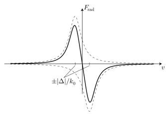
For small velocity  $[v \ll \max(|\Delta|, \gamma)/k]$ , we can expand to lowest order in v to obtain the viscous damping ("friction") force:
