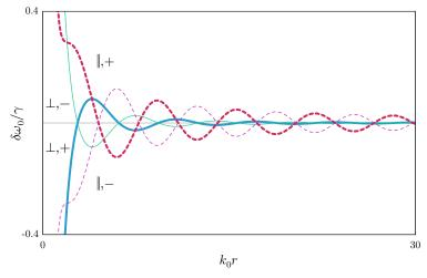
For the frequency (energy) shift, we can see that for small distances and in-phase dipoles, the perpendicular (z-z) orientation produces an attractive potential, while the parallel (x-x) orientation produces a repulsive potential, as we expect for static dipoles.
