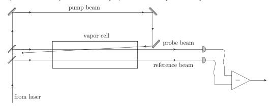
Three beams are split from a common laser source. Two probes are sent through the cell. The third beam acts as a pump, and nearly counterpropagates with one of the probe beams, producing the Lamb dips. The other probe acts as an unsaturated reference, so that the Doppler profile can be subtracted from the Lamb-dip signal. The saturation spectrum is shown in the following plot.
