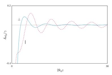
This effect can be interpreted as an ac Stark shift of the atom due to its own radiated field. Note that only the parallel component has a radiative (1/z') component. In the near field, the frequency shift becomes very large until the dipole approximation breaks down. The decay rate has similar oscillatory behavior, but the prediction is not divergent as the atom approaches the wall.
