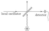
Even though this setup detects some "irrelevant" light due to the local oscillator, the amount of information that we acquire via this setup (within the idealizations below) is equivalent to that of direct detection. If the
