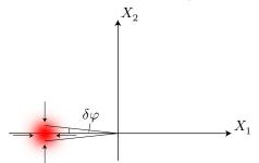
The price of this "omnidirectional" phase sensitivity is that the phase uncertainty decreases (assuming the decrease to be dominated by the measurement information) at half the rate for the best case of homodyne detection. Of course, it greatly outperforms the homodyne measurement in its worst case, and the heterodyne measurement simultaneously provides information about the field amplitude.
