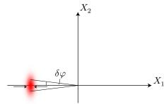
Thus, gaining information on the phase in homodyne detection depends on having a particular phase to begin with. That is, the phase sensitivity of homodyne detection has a phase-dependent sensitivity. Heterodyne detection has the advantage that the measurement reduces the phase uncertainty for any phase, since as we saw above, the uncertainties of *both*  $X_1$  and  $X_2$  decrease in response to the measurement.
